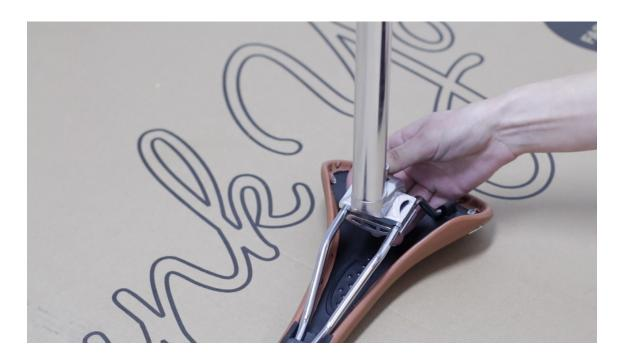
Insert the seat post into the frame. We left it at half a height, and without letting go of the seat post, tighten it with the ALLEN wrench.
