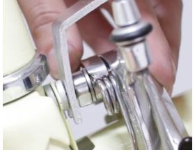
Finally, we introduce the lateral supports in the front bushing
